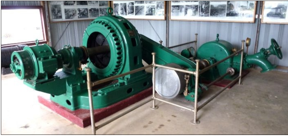
The first hydro plant, with 2 nd governor, on display in a museum shed at Batlow.
