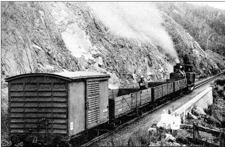
An Abt locomotive pushing a rake of goods wagons up the Razorback incline – in the early 20th century. The concrete wall (lower right) is the only remnant of the line still existing. Image: CAPCOL Collection.
