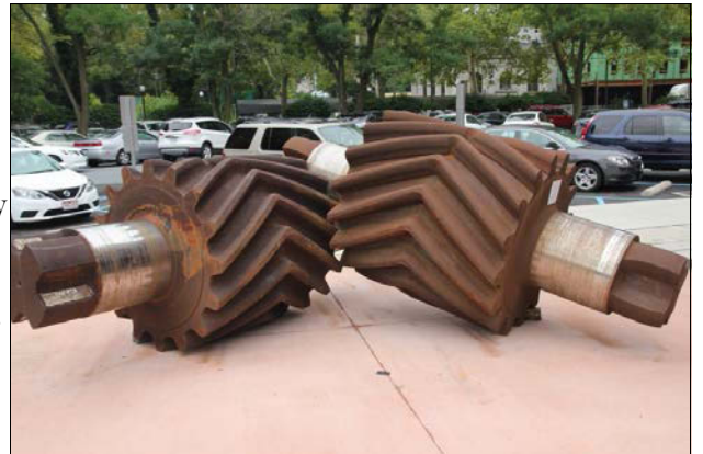
Image above: A pair of double helical pinion gears at the National Museum of Industrial Heritage, artistically posed. The principle was pioneered by André Citroën. These were once meshed & drove a rolling mill. Look for the badge on the next Citroen car you see!
