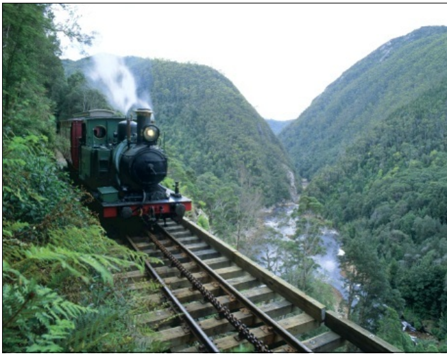
The West Coast Wilderness Railway, and one of the original Abt locos. Source - EHTasmania.
