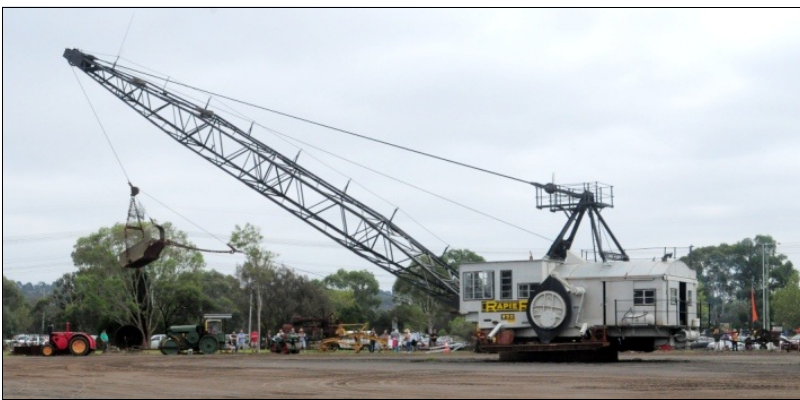
The Ransomes & Rapier walking dragline – out for a stroll. Photo Owen Peake.
