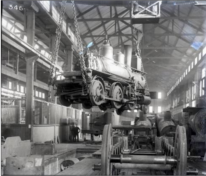
Steam loco "Major" brought in for repairs after a rear-end collision in 1914. From Thompsons Archives.
