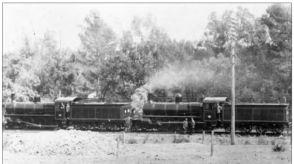
Two of the many Dd steam locomotives built by Thompsons for the Victorian Railways from 1913. These two new locos are in the railway siding at Thompsons, waiting to go. Ph. Thompsons Archives.
