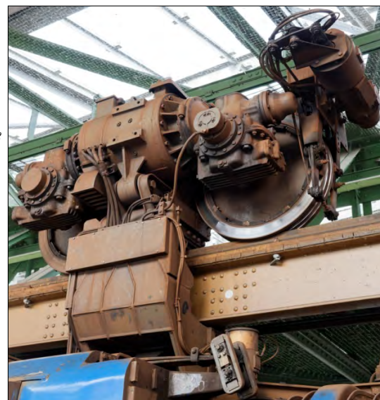
Detail of a suspender, motor, worm gears, wheels & brake (top right) of a GTW 72 carriage.
