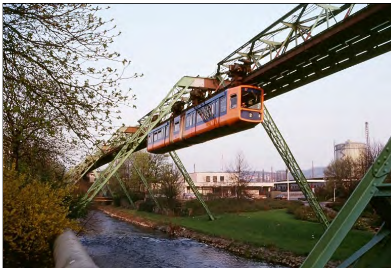
Die Wuppertaler Schwebebahn and the River Wupper in 1992. The original passenger cars were joined together by chains, allowing them to traverse very tight bends. The modern cars are joined like Sydney’s bendy-buses, with a concertinaing cladding down the sides and at top and bottom. Photo: M Doring, 1992.
