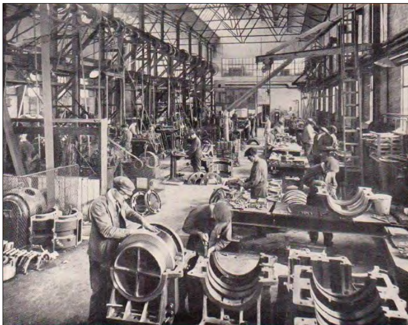
Early days at the Newcastle UK Michell works, showing the production line for the Thrust Bearings. Image printed in a 1920s Michell Bearings catalogue. Source: Stephen Phillip.
